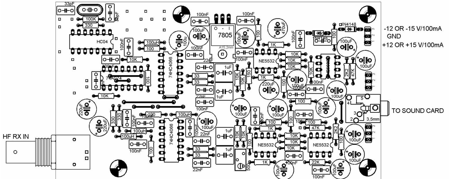
DR2A++ parts placement for internal crystal fundamental mode oscillator to 30 MHz or 3 overtone mode oscillator typical case  $Q=28322\text{kHz}$  (reduce 100K in HC04 feedback to 4k7)
